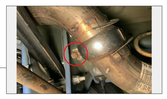
Using a jack and jack stands, raise and support the vehicle off the ground. Loosen the (1) ball clamp on the rear of the muffler using a 13mm socket. Repeat the process for both sides.
