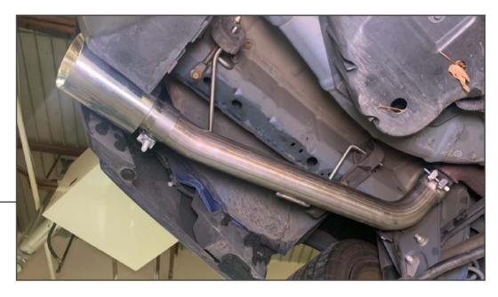
Slide the new ball clamps onto the over-axle pipe loosely, and put the muffler delete pipe into the hanger closest to the rear bumper on each side. Tighten the exhaust hanger bracket to the vehicle using the original 13mm bolts.
