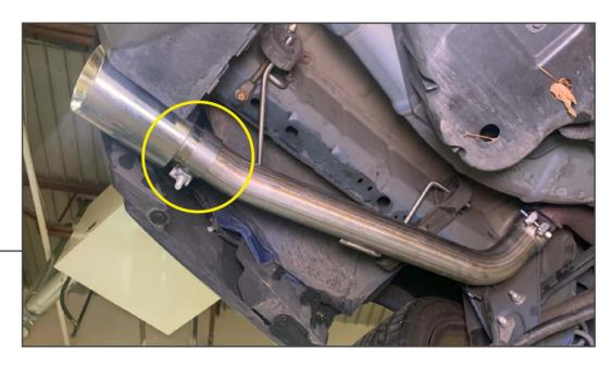
Install the exhaust tip using (1) provided band clamp per side, tighten using a 13mm socket and torque to 42 ft/lbs.
