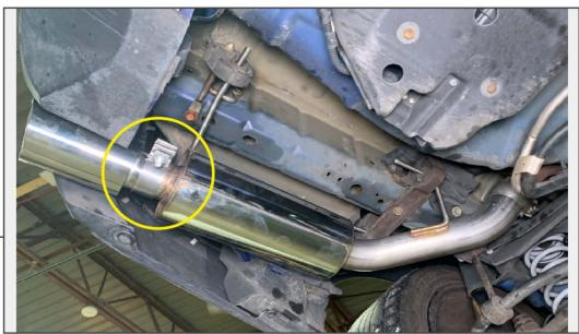
Install the exhaust tip using (1) provided band clamp per side, tighten using a 13mm socket and torque to 42 ft/lbs.
