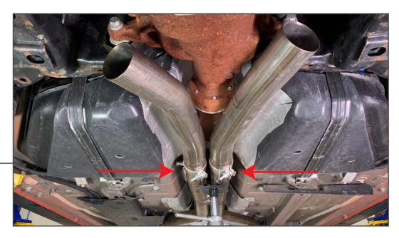
Attach the mid-section pipes to the X-Pipe using provided 3" exhaust clamps. Do not tighten the clamps.
