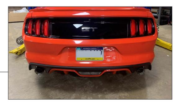
When both mufflers are attached to the vehicle, align the pipes until the fitment to the rear bumper is even on both sides. Tighten all exhaust clamps.
