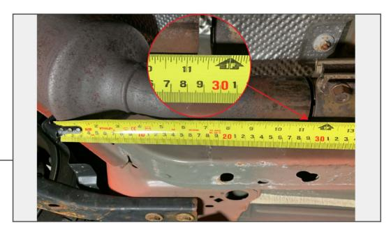
Measure back 11.25" from the lower casing on the catalytic converter on both sides, and leave a guide line using a permanent marker. Support the rear of the exhaust, and cut along the marked areas.
