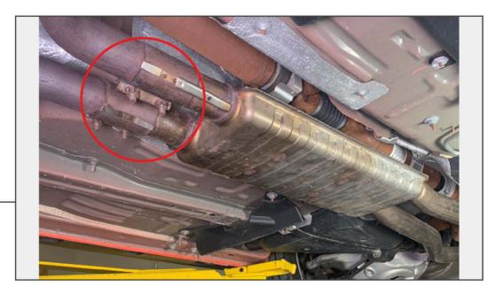
While supporting the exhaust, loosen (2) exhaust clamps on the front of the resonator and slide the clamps aside.
