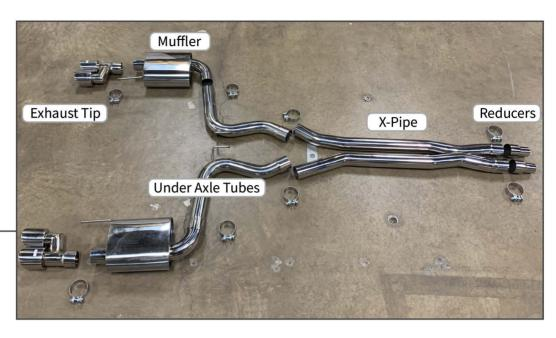
Lay out the new exhaust as shown. (15-17) Vehicles will utilize the single tips. (18-20) Vehicles will use the dual tips. Transfer the exhaust hangers to the new exhaust system.
