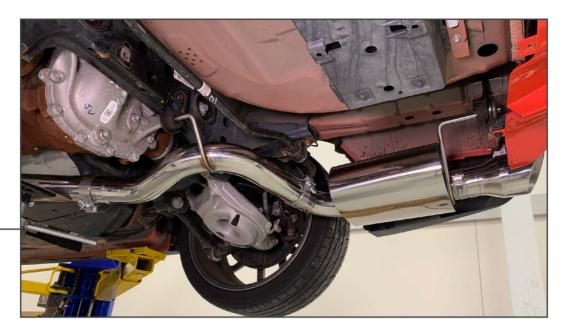
Loosely connect the under axle tubes and mufflers. Then, install the muffler and axle tube assembly onto the x-pipe. Loosely install the exhaust tip and adjust for best fit. Re-install the factory exhaust hangers using the factory hardware.
