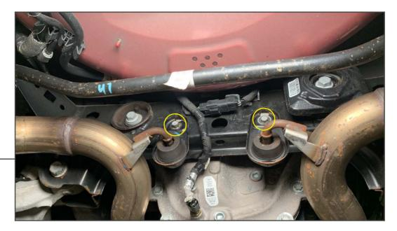
Remove the (3) 13mm bolts securing the exhaust hangers to the rear sub-frame. Unhook the hangers from the sub-frame.
