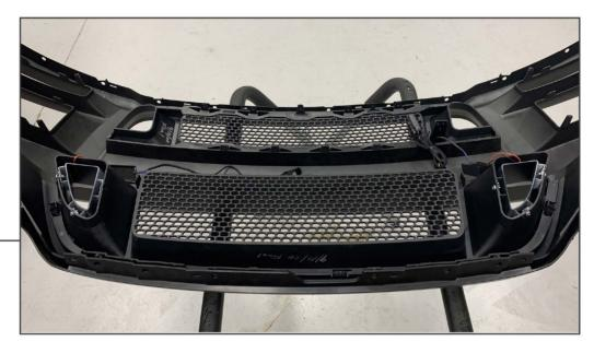
Install the new grille(s) into the bumper by aligning the clip locations with the factory holes. Firmly press the grille through the bumper. You will hear it snap into place.
