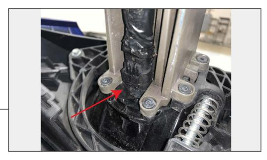
Unplug the fog light harnesses from the fog light housings. Remove bumper from vehicle and place on a soft surface for grille disassembly.
