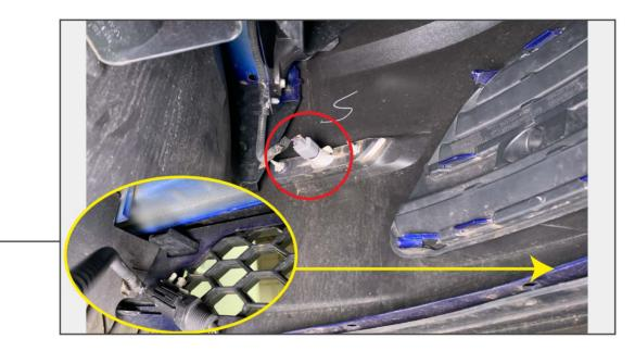
Unplug the turn signal connectors from each side of the bumper. Behind the face of the bumper, remove the sensor from the grille by pulling it down, away from the bumper.
