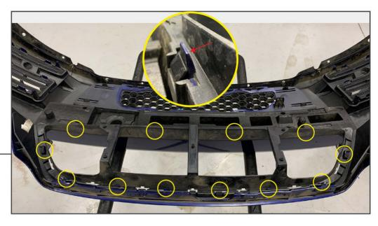
Using a flathead screwdriver, pry back on the clips on the inner layer of the grille.
