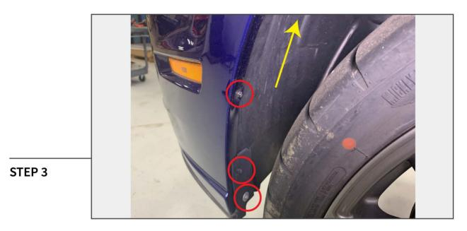
Remove (3) 7mm bolts and (1) Phillips push clip per side.
