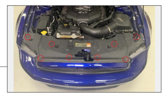
Using a panel removal tool, remove (8) push clips from the radiator cover. Lift radiator cover and set aside.
