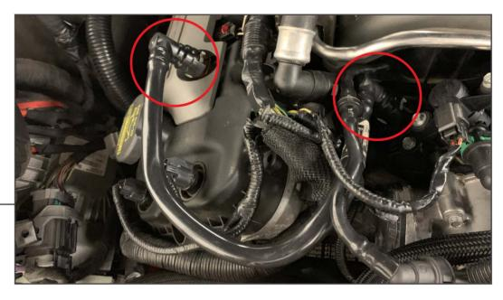
Locate the PCV hard-line circled above. Rotate the gray clip and pull the fittings away from the intake manifold and valve cover.
