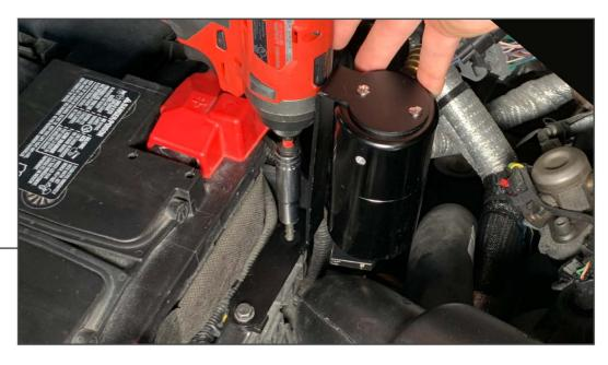
Install the provided clip nuts into the battery tray. Using the provided M6 hardware, secure the catch can to the battery tray.
