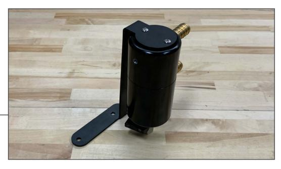
Install the 4 hole mounting bracket to the catch can using the supplied M4 Allen screws so that the mounting tab and barb fittings are facing away from each other.
