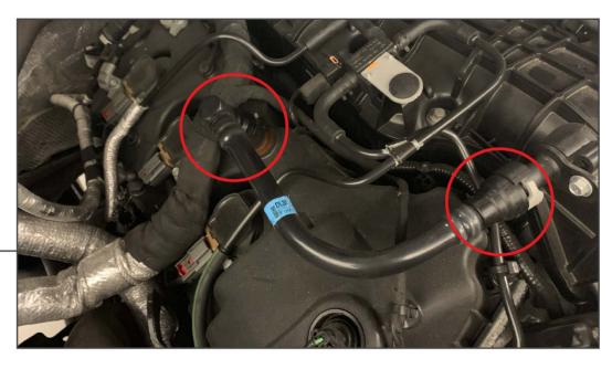
Locate the PCV hard-line. This will very between models and engine sizes but they will always be connected to the valve cover and intake manifold. Rotate the gray clip and pull the fittings away from the engine.
