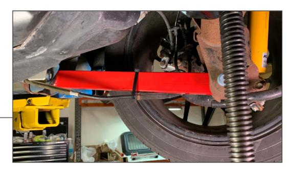
Reattach the emergency brake cable in reverse order. Zip tie the cable to the lower control arm as shown. Repeat the process on both sides and then torque all hardware to 129 ft. lbs. Grease the control arms every oil change.
