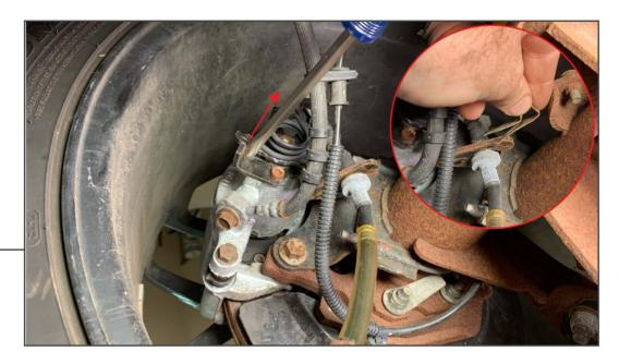
Using a screw driver, pry up on the emergency-brake lever and remove emergency brake cable from the caliper. Pull the retaining clip from the cable bracket and remove the cable from the bracket. Feed the cable through the control arm.
