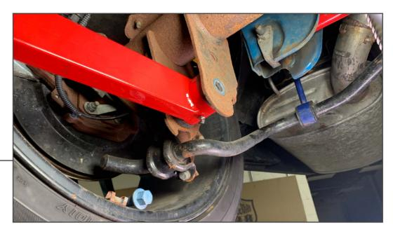
The offset portion of the lower control arm needs to face the center of the vehicle. This needs to be identified prior to step 6.
