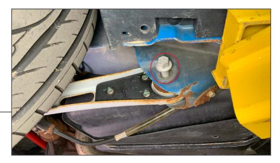
Using a 18mm socket, remove the front bolt.
