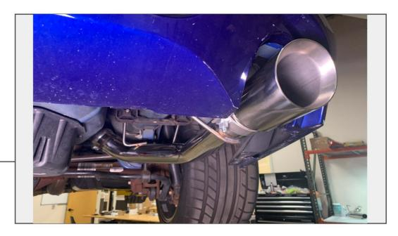
Install the exhaust tip using (1) provided band exhaust clamp per side, tighten using a 13mm socket.
