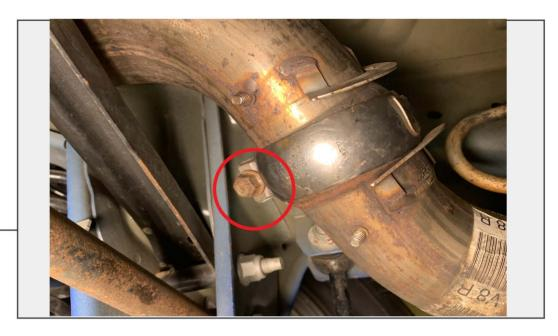
Loosen the (1) ball clamp on the rear of the muffler using a 13mm socket wrench. Repeat the process for both sides.
