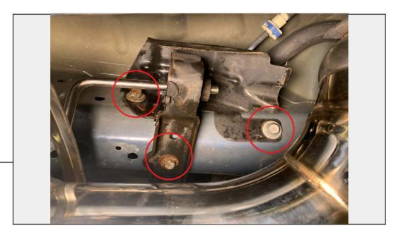
Loosen the 13mm bolts holding the top hanger bracket to the vehicle to release the muffler from the vehicle.
