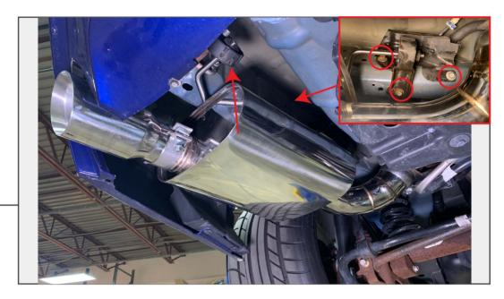
Slide the new ball clamps onto the over-axle pipe loosely, and put the muffler into the hanger closest to the rear bumper on each side. Tighten the exhaust hanger bracket to the vehicle using the original 13mm bolts.
