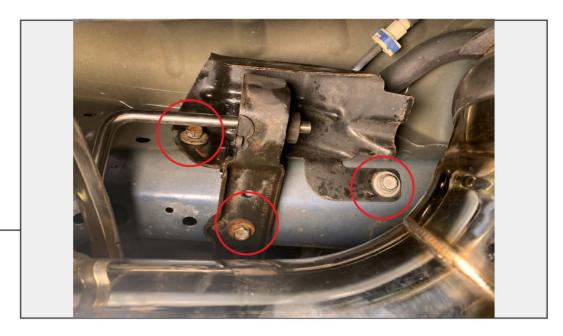
With a helper holding the muffler, loosen the 13mm bolts holding the top hanger bracket to the vehicle to release the muffler from the vehicle.
