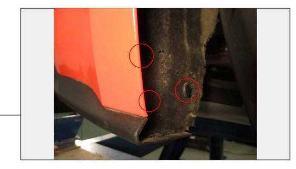
Raise and support the rear of the vehicle with a jack and support with jack stands. Remove the (3) plastic push clips that secure the fender liner to the bumper, repeat on both sides.
