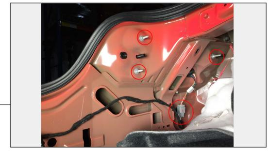
Fold back the inner trunk liners to access and remove the (3) nuts securing the tail lights to the vehicle. Unclip the electrical connections and remove the lights.
