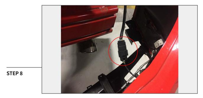
On the right hand side, locate and unplug the bumper wiring connection. Remove the bumper and place it on a soft surface.
