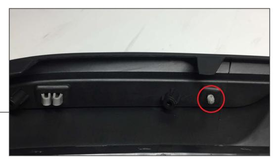
Using 10mm socket, remove the nut securing the rear bumper reflectors. Install the supplied reflectors using the factory nut.
