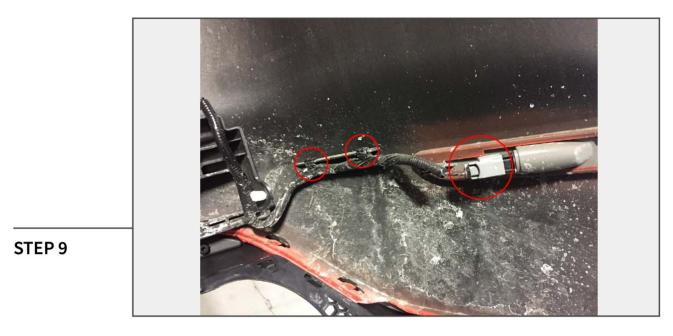
Unplug and unclip the rear bumper lights. Transfer the light to the new bumper.
