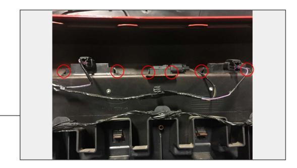
Unclip the license plate light housing and trunk button. Transfer them to the new bumper.
