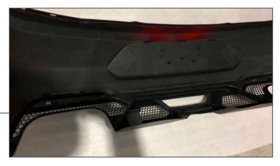
Install the rear valance/diffuser on to the bumper. Firmly press the valance/diffuser into the bumper. The parts will "click" together when properly install.
