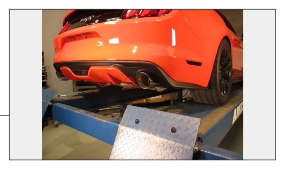
Remove the (2) 7mm screws securing the bumper to the bottom bumper bracket.
