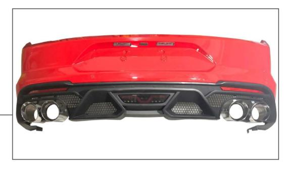
Clip the bumper on to the vehicle. Test the lights prior to reinstalling the bumper in reverse order. Ensure the electrical connection removed in Step 8 doesn't get pinched between the metal and the bumper otherwise the bumper will not fit correctly. Installation is now complete.
