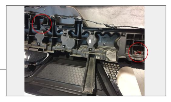
Unclip the rear bumper brace from the bumper. \*\*If equipped, unplug and removed the backup sensors to the new bumper.
