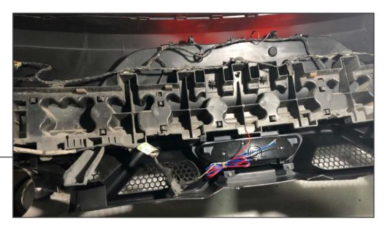
Then clip the bumper brace and wiring harness on to the bumper. Ensure electrical connector are plugged in.
