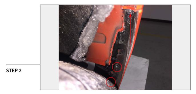
Fold the fender liner back to access the (3) 7mm bumper cover screws. Repeat this process on both sides of the bumper.
