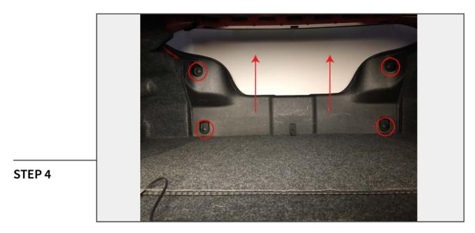
Remove the trunk trim panel by unscrewing the (4) cargo net fasteners. Pull the trim panel up and away from the vehicle.
