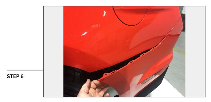
With the fasteners and tail lights removed, carefully pull the bumper cover away from the vehicle.
