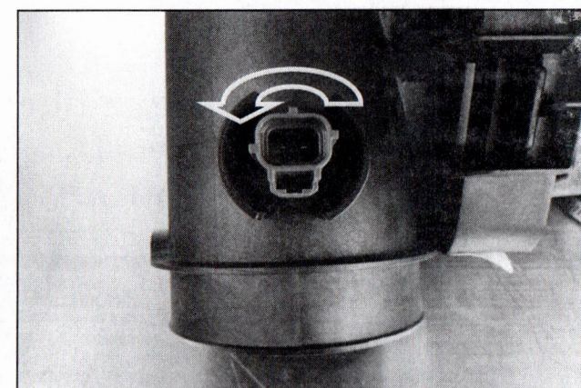
8. Tilt the air temp sensor rearward so the locking tab clears the ramp and rotate it counterclockwise 1/4 turn to release it.
