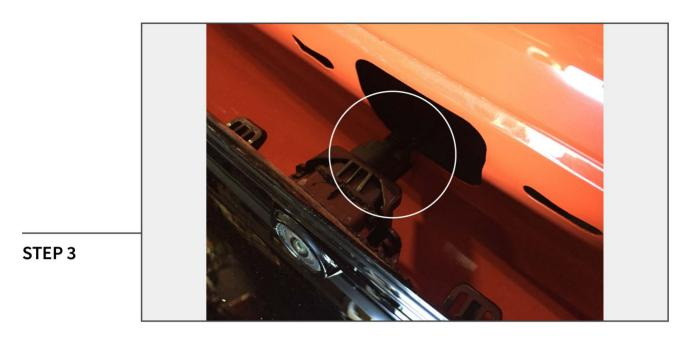
Unplug the reverse camera. Then remove the panel from the vehicle.
