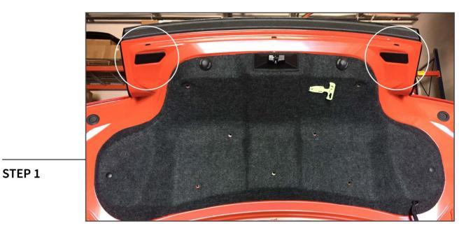
Using a panel removal tool, remove the caps covering the deck lid panel bolts. Then, remove the (4) 7mm screws.
