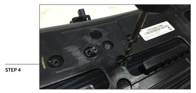
Remove the deck lid emblem by slowly/carefully removing the plastic weld from the back of the deck lid panel. Use an oversized drill bit and only remove enough material so that you can remove the emblem.
