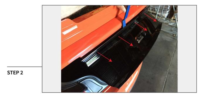
Use the panel removal tool to gently separate the factory deck lid panel from the deck lid.
