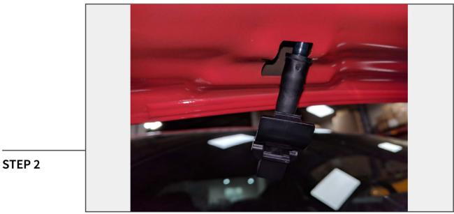
Locate the Squirter nozzles, and remove by carefully prying away from the hood and disconnecting the hose.
