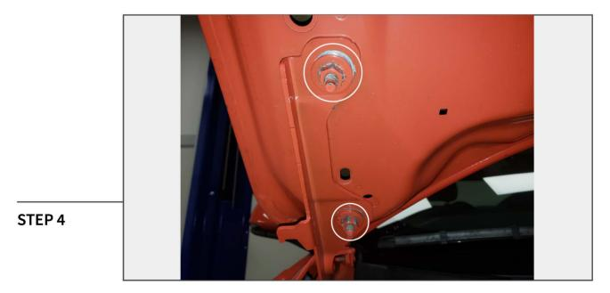
With a helper, carefully remove the (2) 15mm hood hinge nuts on both sides of the hood. Place the hood on a soft padded surface so that you can easily access the underside of the hood.
