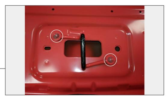
Remove the factory hood latch by removing the (2) 10mm nuts.
