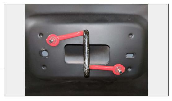
Install the hood latch to the new hood using the factory 10mm nuts.
