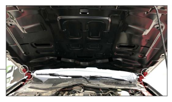
With a helper, install the hood using the factory (4) 15mm nuts. Be sure to properly align the hood with the fenders of the vehicle. You may have to repeat this a few times to achieve desired fitment. Then reinstall the windshield washer fluid line, and nozzles. \*\*Note: Be careful opening and closing the hood when aligning for proper fitment so damage does not occur to the paint.
