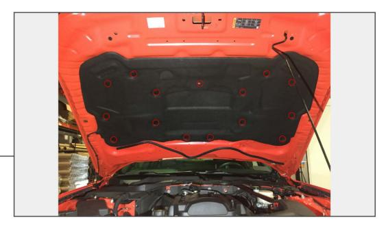
Begin by raising the hood to gain access to the under hood insulation. Remove the (15) push pins that hold the insulation liner to the hood.
