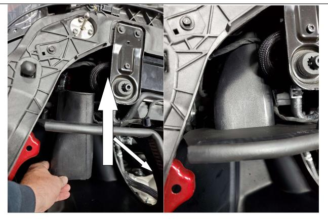
Line up duct on to the factory fresh air inlet and slide over.
