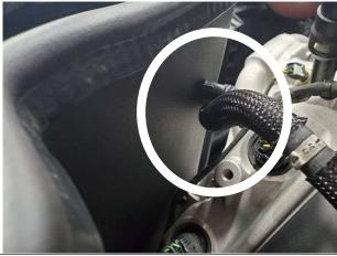
Remove the IAT sensor from the stock intake tube by twisting counterclockwise, roll down O-ring and insert into the grommet in the JLT tube.
