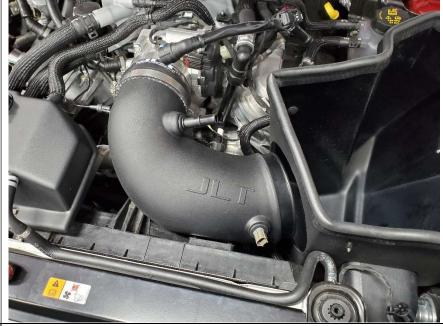
9 Install the air filter, tighten all clamps and plug in IAT, PCV and Vacuum connections.
