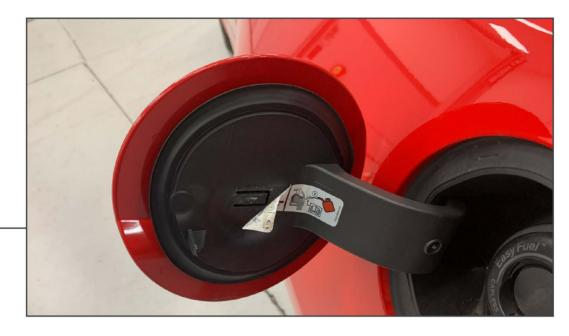
Open the fuel door. Carefully peel back the warning stick to expose the fuel door clip.
