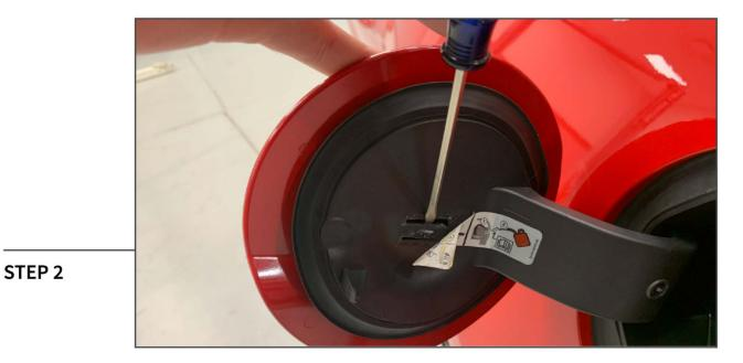
Using a small flat blade screw driver, gently pull open the clip.
