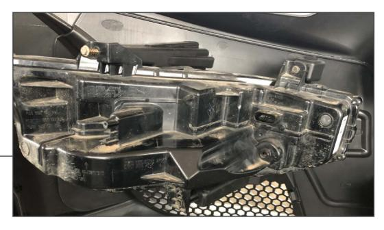
Transfer the factory turn signals from the original bumper onto the new bumper using the factory hardware.
