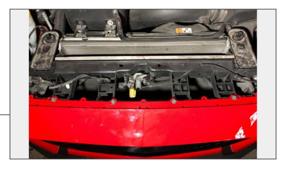
Install the new bumper onto to vehicle following Steps 1-7 in reverse order.
