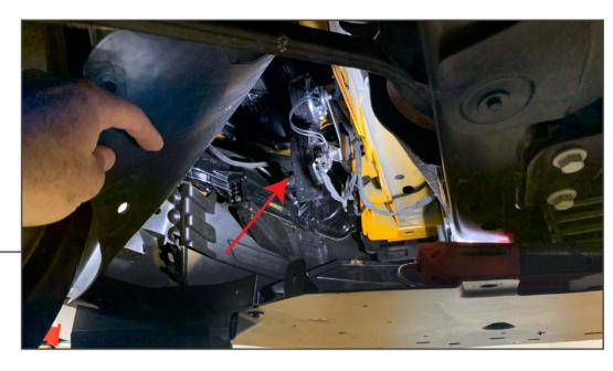
Fold back the fender liners to access the turn signal plugs (1) on each side. Depress the electrical connector's retaining clip and pull the plug away from the light.
