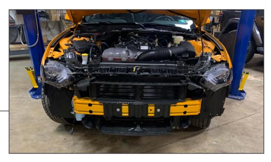
Remove the bumper and splash shield as an assembly from the vehicle and set it to the side.
