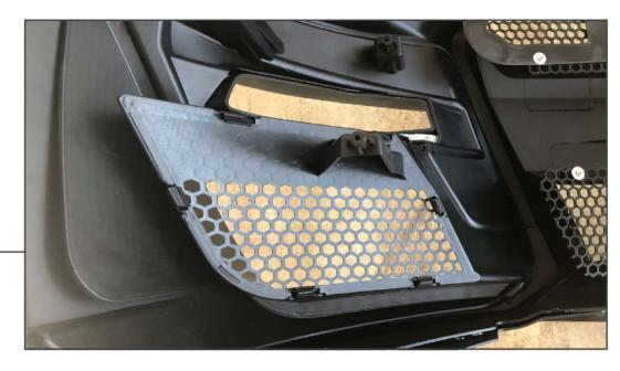
Remove the turn signal bracket from the bumper using a 7mm socket.
