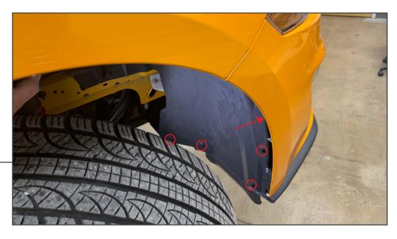
Remove the (3) push clips on the outer edge of the inner fender liner and the (2) at the bottom of the splash shield from each side of the bumper.
