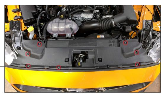
Raise and support the vehicle to gain access to the under side of the bumper and rocker panels. Using a soft pry tool, remove the (8) plastic push clips securing the radiator cover to the vehicle.
