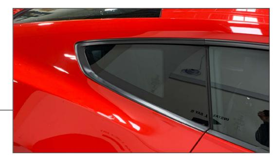
Begin the installation by thoroughly cleaning the quarter window glass with automotive grade soap and water. Allow the window time to fully dry. \*\*Recommended: Wipe the glass down with isopropyl alcohol to ensure the glass clean and free of any contaminants.
