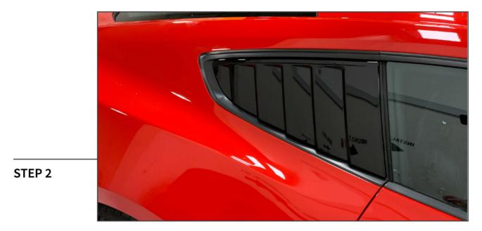
Test fit the part on the window to become familiar with how the louver fits.
