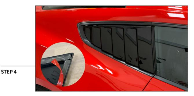
Peel back the tape backing and install the quarter window louver to the vehicle. Apply firm even pressure on all tape ledge locations to ensure proper adhesion. Installation is now complete.
