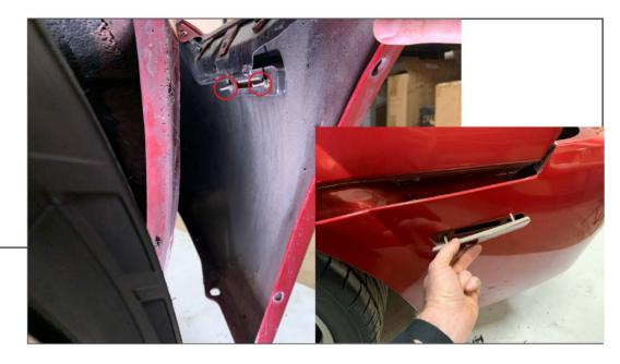
Using a 10mm deep socket, remove the (2) nuts securing the factory reflector to the vehicle. Then remove the reflector from the vehicle.
