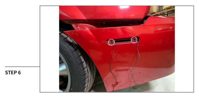
Align the LED reflector with the bumper. Then feed the green and black wires through their respective mounting holes.
