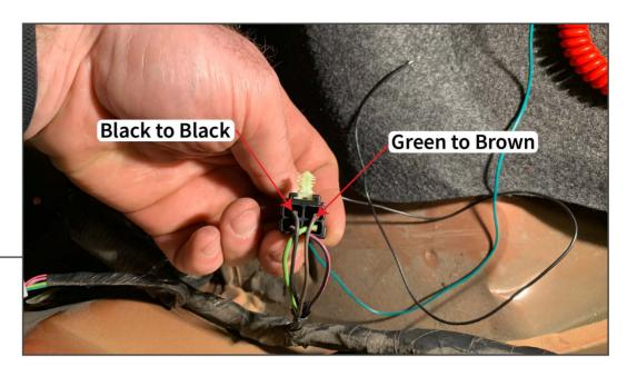
Using the suppled Scotchlok connectors connect LED reflector wiring to the factory tail light harness.
