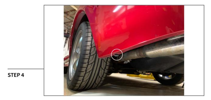
Using a pry tool, remove the push clip on the bottom of the bumper.
