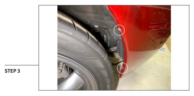
Remove the (2) Phillips head screws on the inside of the wheel well.
