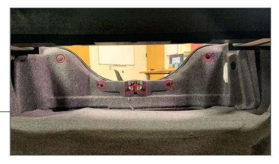
Using a pry tool, remove the (6) plastic push pins securing the trunk trim to the vehicle. Remove the trim from the vehicle.
