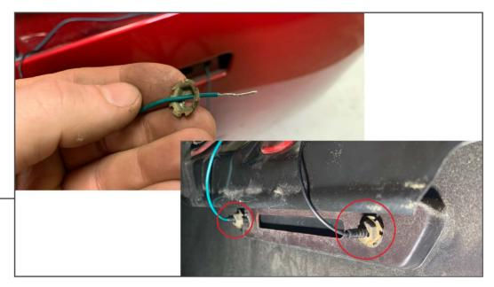
Slide the original nuts over the wires as shown. Secure the LED reflector to the bumper by tightening the nuts using a 10mm wrench.
