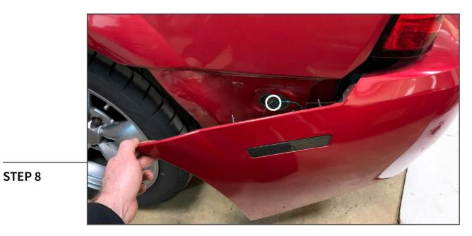
Using a razor blade, cut a small hole into the body grommet behind the LED reflector. Insert the wiring through the body grommet. Feed the wiring up to the tail light wiring connector.
