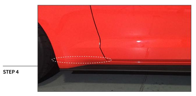
Pull the front edge of the rocker panel away from the fender. The rocker panel is clipped in across the top edge.
