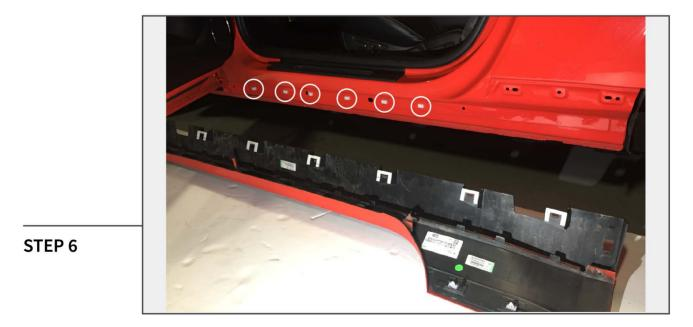
Once the top (3) clips are removed, gently pull down on the rocker panel to access the remaining clips. \*\*Note: The panel may pull away from the panel leaving the clips in the rocker panel. The clips will need to be removed in order to reinstall the new rocker panel.
