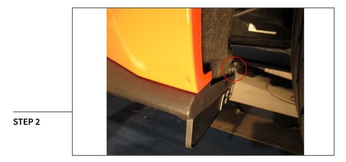
Remove the push clip securing the fender liner to the rear rocker panel. This clip will not be reused.
