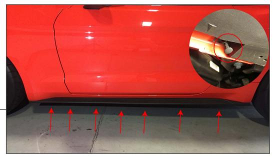
Remove the (7) push clips holding the rocker panel to the underside of the vehicle.
