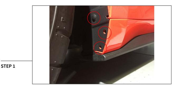
Remove the (3) push clips holding the inner fender liner to the rocker panel.
