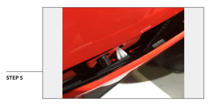
Using a soft pry tool, gently pull the rocker away from the rear quarter panel. Depress the sides of the (3) white clips to release them from the vehicle.
