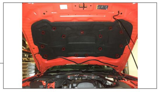
Begin by raising the hood to gain access to the under hood insulation. Remove the (15) push pins that hold the insulation liner to the hood.
