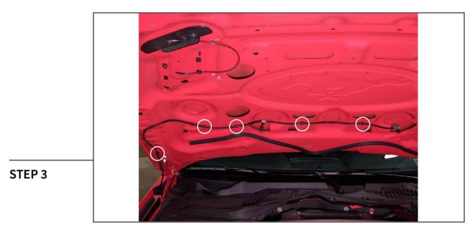
Using a trim panel removal tool, remove the (5) push clips holding the windshield washer line to the hood.
