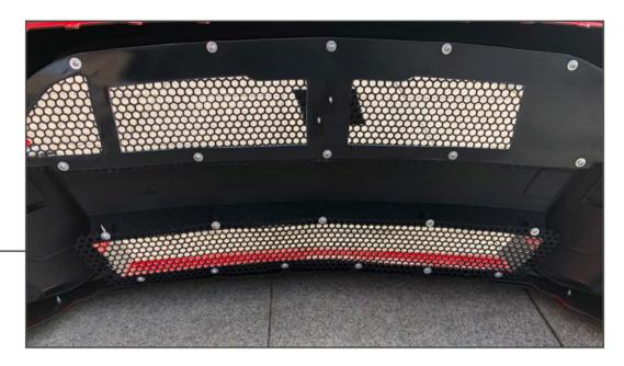
Install the upper and lower grilles using the (28) provided 15mm self-tapping screws and flat washers.
