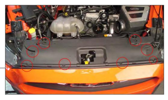
Jack the vehicle up and support the font end with jack stands. Using a trim panel removal tool, remove the (8) push clips securing the radiator cover remove it from the vehicle.
