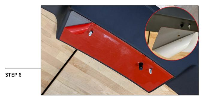
Ensure the middle mounting surface is clean and dry. Peel back the white tape backing and install the die cut tape pad to the spoiler.
