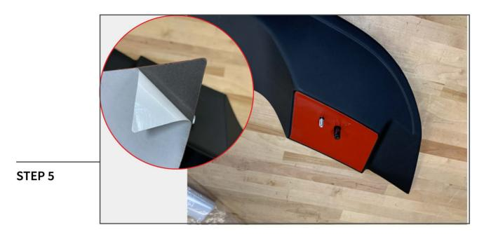
Ensure the outer mounting surfaces are clean and dry. Peel back the white tape backing and install the die cut tape pad to the spoiler.
