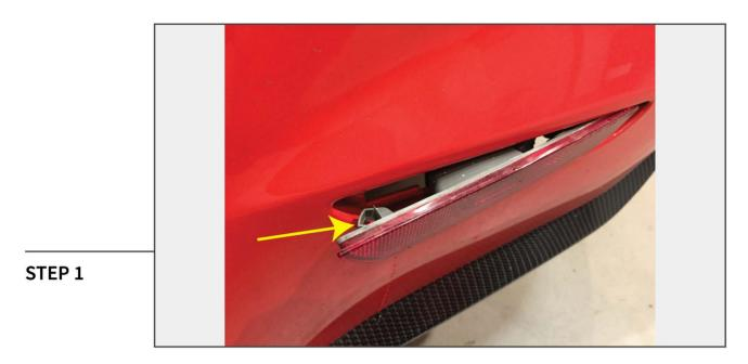
From below, reach behind the bumper cover and depress the clip on the front of the light.
