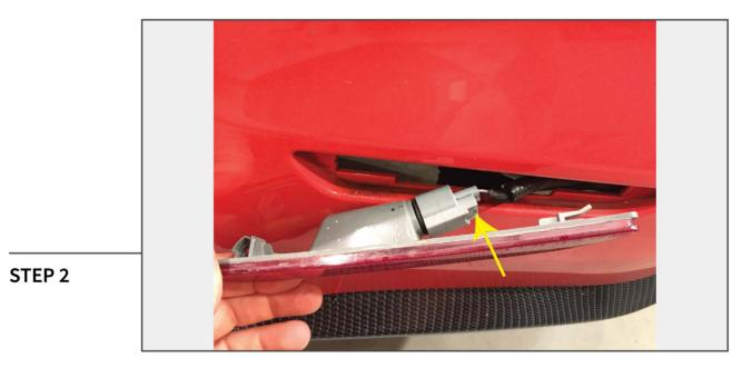
Depress the wiring harness plug to remove the light from the vehicle.
