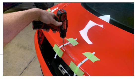
Once the spoiler is removed, carefully drill the center of the template holes. Finish with a 1/4" drill bit. Use clear touch up paint to cover any exposed metal to prevent rusting.
