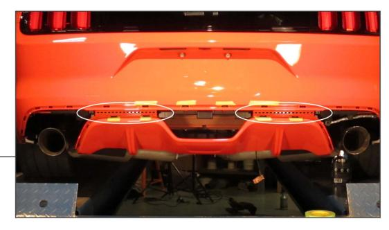
Once the lower trim panel is removed from the bumper, the factory diffuser will need to be cut from the bumper. Do this by cutting along the dotted lines shown above.
