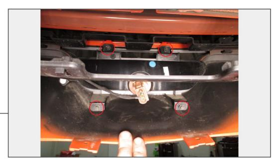
Disconnect the reverse light plug. Gently pull the bottom of the bumper down to access the (4) 7mm screws securing the 3rd brake light to the bumper. Remove the light from the vehicle, reverse light and hardware will be reused.
