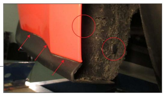
Support the rear of the vehicle so you can access the underside of the bumper. Remove (2) fender liner clips, on each side, to gain access to the (3) 7mm bolt holding the lower bumper trim to the bumper.
