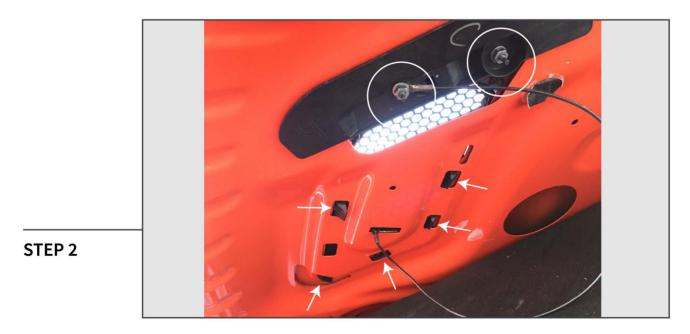
Remove the (2) 9mm nuts holding the factory vent in place. Then, using a small flat head screw driver, depress the vent clips on the underside to remove. It is important to hold the vent while releasing the clips to prevent the vent from popping out unexpectedly and scratching your hood.
