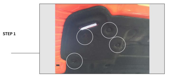
Remove the hood liner push pins and hold back the liner to gain access to the factory hood vent mounting nuts.
