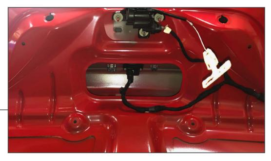
Remove the (9) push rivets, (2) rubber bumpers, and trunk latch trim to remove the trunk lid liner. Once the liner is removed you will have access to the (2) remaining clips holding the decklid panel and the reverse camera wiring harness. Release the clips, unplug the harness, and remove the decklid panel from the vehicle.
