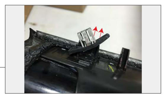
Using a flat head screw driver, remove the metal clips from the factory decklid panel and reinstall them on the Saleen decklid panel.
