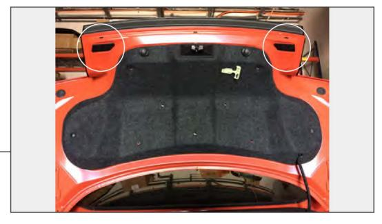
Using the Trim Panel Removal Tool, gently remove the caps covering the decklid panel bolts. Remove the (4) 7mm bolts, taking your time so they don't accidentally fall between inner and outer layers of the panel.
