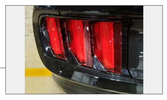
Wash the taillight with soap and water and dry thoroughly. Clean the inner taillight section with the supplied alcohol pad to remove any remaining contaminants. Once dry, treat the same section with the supplied adhesion promoter.
