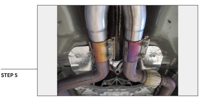
Secure the resonator delete pipe to the vehicle using the factor clamps.
