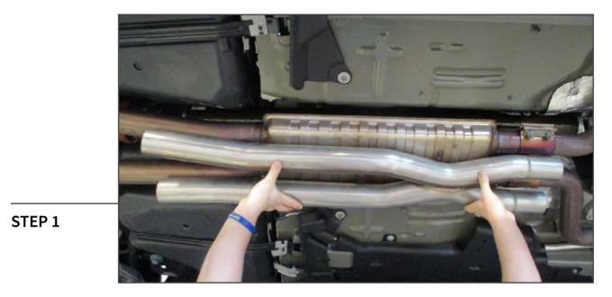
Raise and support the vehicle to gain access to the factory resonator.
