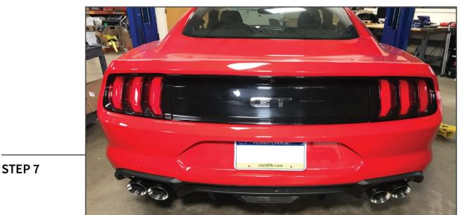
Adjust the tip location by sliding the delete pipe on or out of the factory exhaust. Additional trimming for the factory exhaust may be required. Once the tips are adjusted torque the exhaust clamp nuts to 42 ft. lbs. Lower the vehicle to the ground, the installation is now complete.
