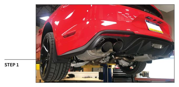
Begin by raising and supporting the vehicle on both sides using a floor jack and jack stands.
