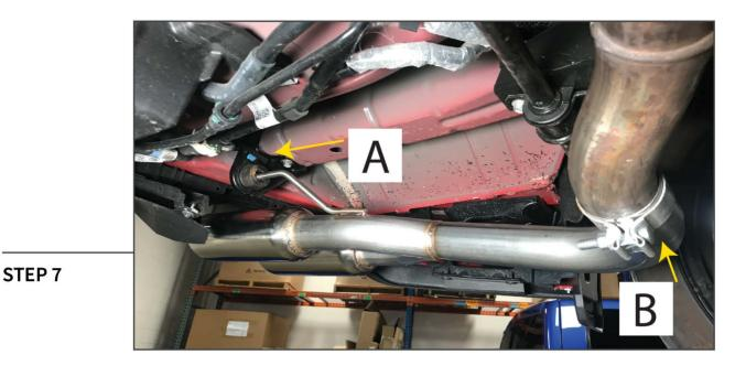
Using the muffler delete pipes, insert the delete pipe hanger into the vehicle's rubber muffler hanger [A]. Then guide the delete pipe into the mid-pipe [B] and secure using (1) provided exhaust clamp. Repeat procedure to opposite side.
