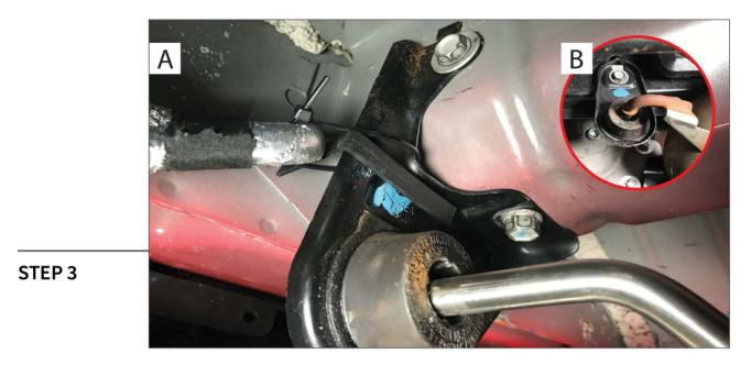
Once loose, move towards the rear of the vehicle and unbolt the (4) exhaust hangers. The muffler hangers [A] use (2) 13mm bolts per hanger, while the remaining pipe uses (1) 13mm bolt per hanger [B].
