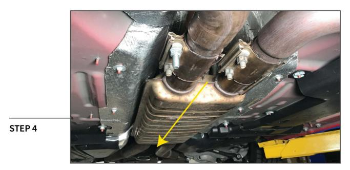
Remove the exhaust from the vehicle. Push the mid-pipe free from the catalytic converter pipes and lift slightly on the rear hangers to free them from the vehicle.
