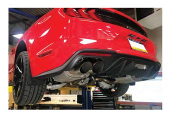
// Step 1: Begin by raising and supporting the vehicle on both sides using a floor jack and jack stands.
