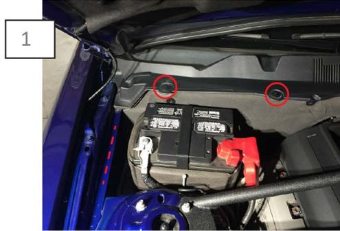
1 Remove the (2) Plastic factory cowl screw clips. Clean the velcro mounting surface on the fender (dashed line above).
