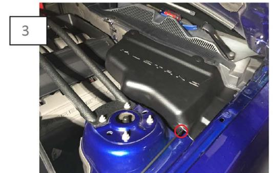
3 Position the part on the car so that the (2) mounting holes line up. Using the supplied push pins, install the battery cover. Place the hood latch cable in the notch. Then apply firm even pressure to the velcro to ensure proper adhesion.
