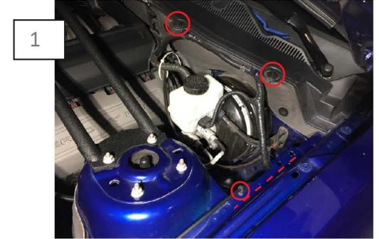
1 Remove the (2) Plastic factory cowl screw clips. Remove the clip holding the hood latch cable to the fender. Clean the velcro mounting surface on the fender (dashed line above).
