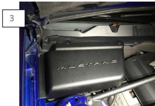
3 Position the part on the car so that the (2) mounting holes line up. Using the supplied push pins, install the battery cover. Then apply firm even pressure to the velcro to ensure proper adhesion.
