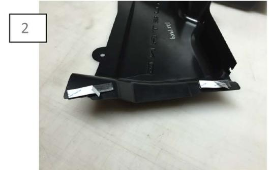
2 Cut the supplied velcro to length. Clean the mounting surface with the supplied alcohol wipe. Allow the part to dry. Then apply the velcro strips. Peel the adhesive backing off the velcro.
