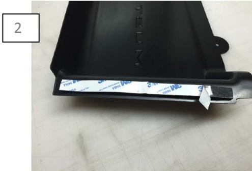
2 Cut the supplied velcro to length. Clean the mounting surface with the supplied alcohol wipe. Allow the part to dry. Then apply the velcro strip. Peel the adhesive backing off the velcro.
