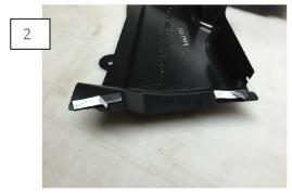
Cut the supplied velcro to length. Clean the mounting surface with the supplied alcohol wipe. Allow the part to dry. Then apply the velcro strips. Peel the adhesive backing off the velcro.
