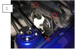
Remove the (2) Plastic factory cowl screw clips. Remove the clip holding the hood latch cable to the fender. Clean the velcro mounting surface on the fender (dashed line above).
