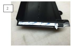
Cut the supplied velcro to length. Clean the mounting surface with the supplied alcohol wipe. Allow the part to dry. Then apply the velcro strip. Peel the adhesive backing off the velcro.
