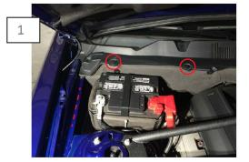
Remove the (2) Plastic factory cowl screw clips. Clean the velcro mounting surface on the fender (dashed line above).
