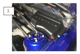
Position the part on the car so that the (2) mounting holes line up. Using the supplied push pins, install the battery cover. Place the hood latch cable in the notch. Then apply firm even pressure to the velcro to ensure proper adhesion.
