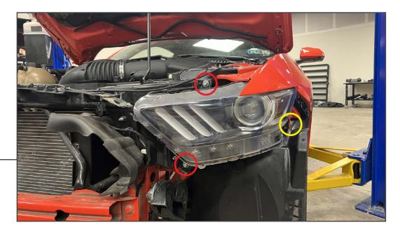
Remove (1) 13mm bolt and (2) 10mm bolts from the headlight assembly. Then, remove the assembly from the vehicle mounting point.
