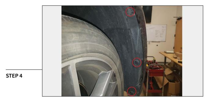
On each side of the bumper, remove the plastic clips holding the fender liner to the bumper.
