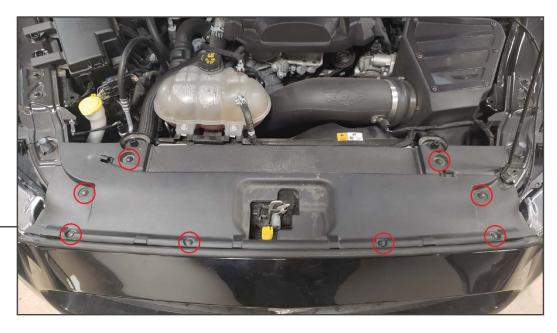
Remove the (8) clips securing the plastic radiator cover to the radiator support and remove it from the vehicle.
