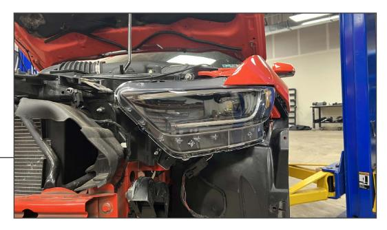
Plug the new headlight into the vehicle wiring harness. Then, secure the new headlight into the vehicle mounting points re-using the original hardware.
