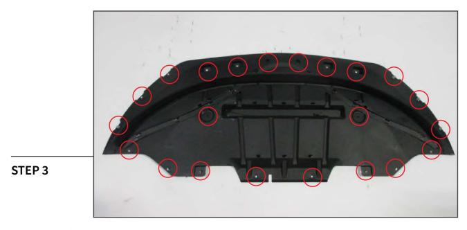
Support the front of the vehicle to access the bumper splash shield.
