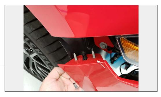
With the (2) 10mm nuts removed from the bumper bracket, you will still need to release the ribbed push rivet before the bumper will separate from the fenders. Take a long extension with a small socket and use that to push downward on the tip of the push rivet, this will push the rivet most of the way out. Gently pull down on the bumper to release the rivet the rest of the way. Remove bumper and set down on a non-abrasive surface where you can easily work.
