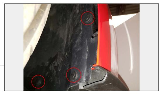
On each side of the bumper, remove the plastic clips holding the wheel well liner to the bumper/splash shield.
