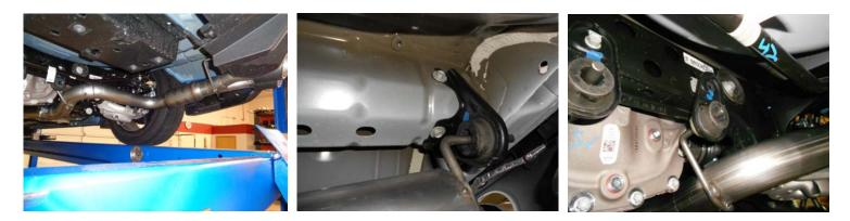
7) Place the right muffler assembly **#815430-513** up into position and slide onto the factory pipe approximately 2½". Support the assembly with a stand and remount the rear hanger mount to the frame and tighten securely. Remount the front hanger to the cross member and tighten securely. Leave the clamp on the inlet loose for now. Repeat this step with muffler assembly **#815430-512** on the left side of the vehicle.
