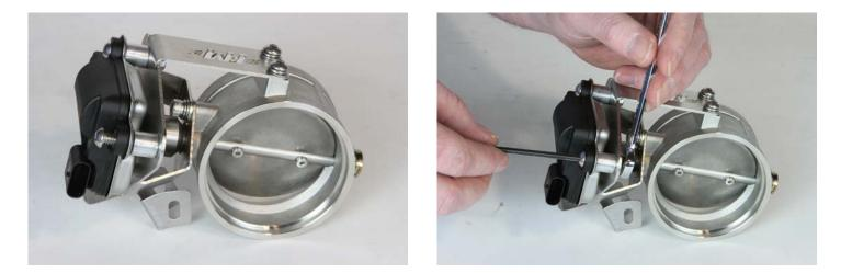
6) Use the remaining  $\frac{1}{4}$ " hardware to secure the actuator to the mount in the remaining two holes. Tighten securely using a 7/16" open end and 5/32" Hex wrench.
