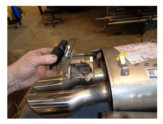
3) Lift the actuator with the heatshield and spring attached from the factory valve assembly.
