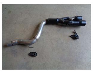
1) Place the new Flowmaster muffler units next to the factory units and swap the front and rear hanger mounts from the stock mufflers to the new mufflers. Also, place a provided 2.50" clamp onto the inlet of each assembly. Tighten the clamp just enough to hold in place.
