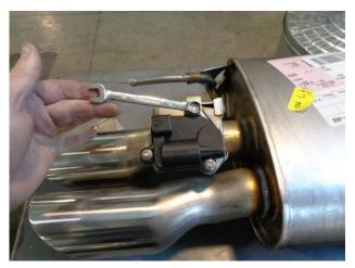
2) On the factory mufflers, use a 10mm wrench to remove the three nuts securing the exhaust valve actuator to the exhaust valve. Place the three nuts and the grounding clip aside for re-installation on the new Flowmaster mufflers.
