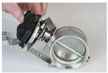
4) **Installing the actuator onto the new valves:** Line up the spring arm with the notch in the valve shaft and lower into place. The holes in the actuator assembly should line up with the holes in the mount, rotate if required.
