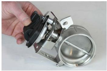
5) Place a supplied 1/4" Button head screw thru the grounding clip removed from the stock valve and then into the hole on the opposite side of the FM in the mounting plate. Place a supplied ½" spacer between the mount and the actuator heatshield, then follow with a supplied lock washer and nut on the bottom side of the mount.
