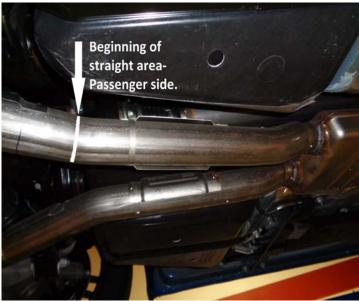
4) Behind the factory center resonator, follow the pipes back just past the second bend of each pipe, make a mark on each pipe where the bend ends and the straight area begins. See above photos. At the rear of each muffler unplug the wire to the factory exhaust actuator and tuck the connection up out of the way until ready to re-connect to the new mufflers.
