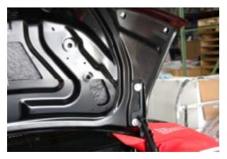
**Step 10:** With the Anderson Composites trunk installed, reinstall the tail light harness, emergency trunk release, bump stops, and if applicable, the tail lights.
