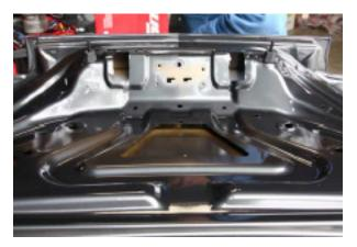
**Step 8:** If applicable, install license plate lights and tail garnish onto the Anderson Composites trunk. (Note: light holes are intentionally made smaller than OEM trunk to ensure a snug fit. To resize, use a file.) Otherwise, proceed to install your OEM latch onto the carbon trunk using your OEM screws, clips, etc. In some cases it may be necessary to enlarge holes to ensure a snug fit.
