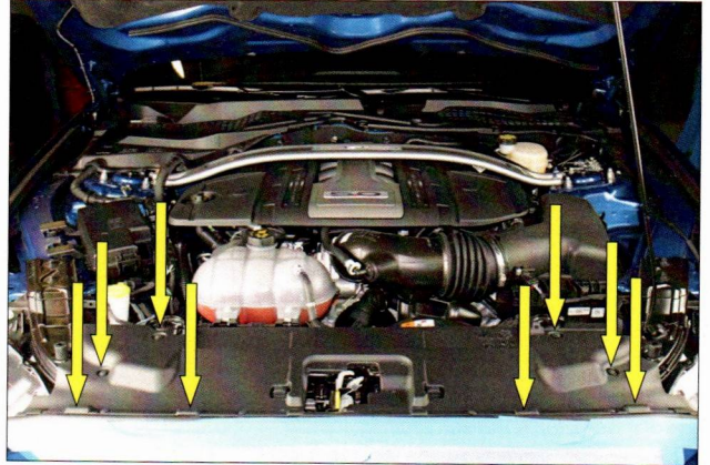
12. Remove the eight plastic rivets in the core support cover and remove the cover from the vehicle.
