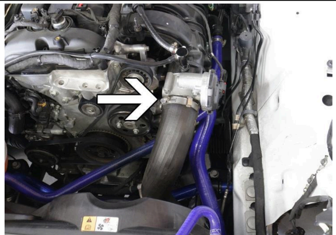
9. Loosen the hose clamp on the throttle body.
