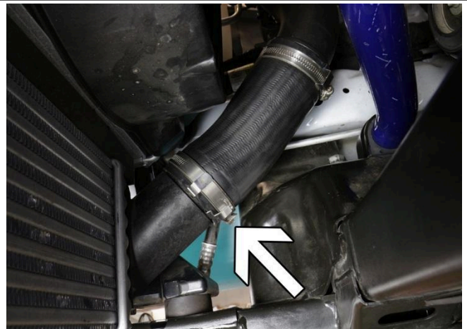
13. Loosen the hot side lower hose clamp.
