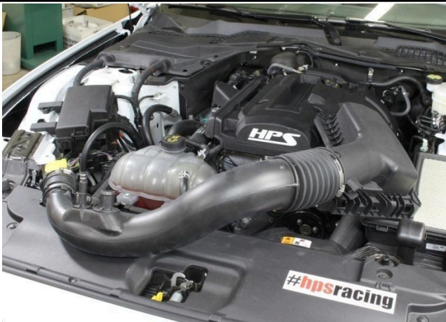
6. Remove the air box and intake elbow from the engine bay.
