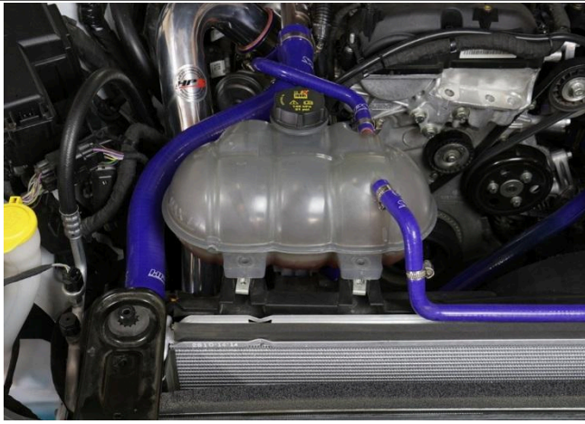
22. Re-install and secure the coolant tank reservoir.
