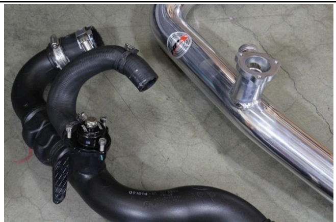
15. Transfer the recirculating hose and the stock bypass valve to the HPS hot pipe.
