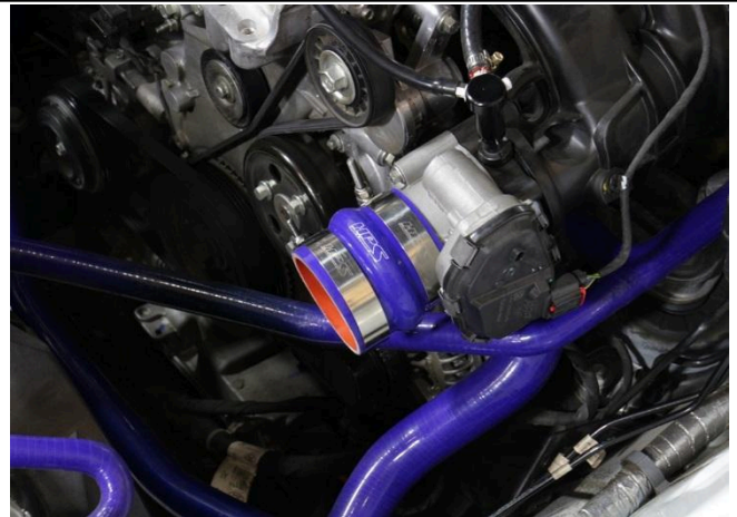
19. Insert the hump coupler onto the throttle body side along with the t-bolt clamps.
