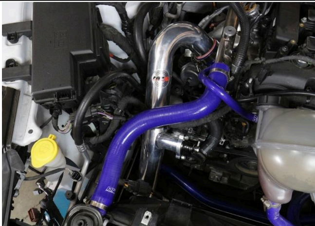
18. Insert and secure the HPS hot pipe into the couplers.
