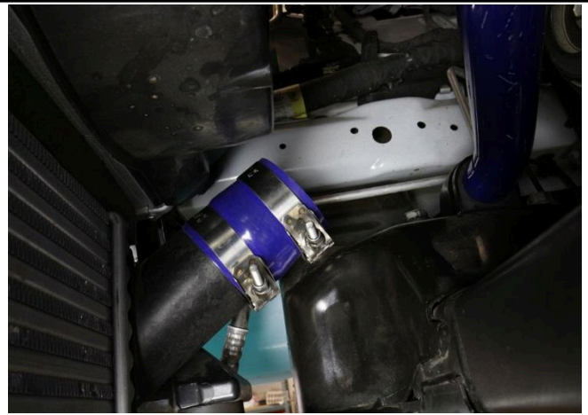
17. Insert the 2.5" coupler onto the intercooler inlet along with the T-bolt clamps.
