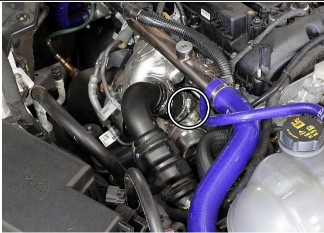
10. Loosen the lower hose clamp that's connected to the intercooler and remove the hose from the vehicle.
