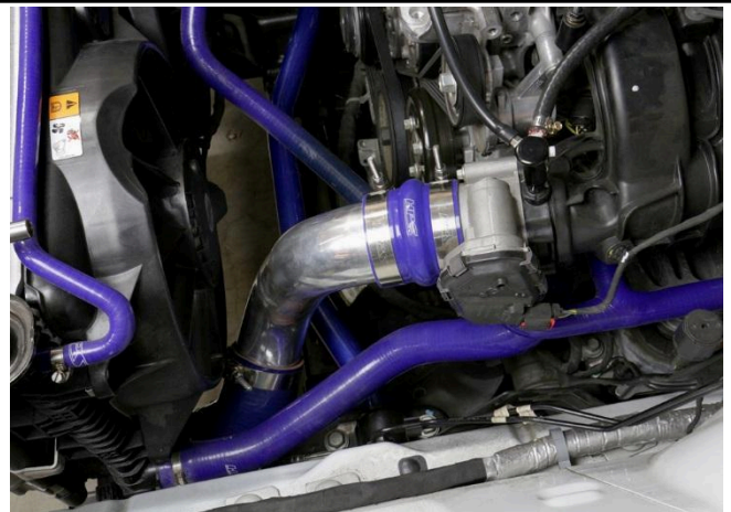
21. Insert and secure the cold pipe into the couplers.
