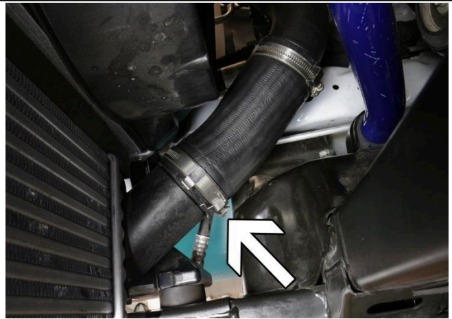
12. Remove the two bolts securing the reservoir and leave it aside to access the other lower hose clamp.
