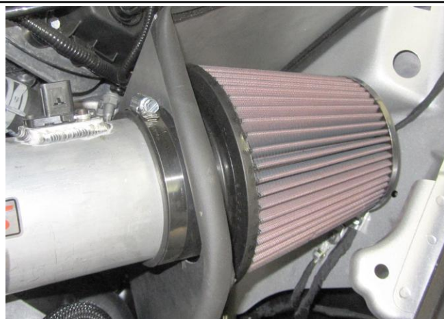
20. Remove the clamp from the HPS air filter and place the clamp onto the intake pipe first, then install the air filter onto the intake pipe.
