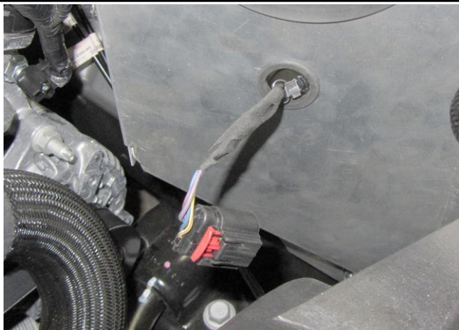
15. Install the rubber grommet and feed the MAF sensor harness through the opening of the heat shield.
