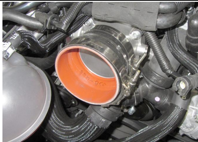
16. Place the reducing coupler and T-bolt clamps onto the throttle body. Only tighten the clamp on the throttle body side for now.
