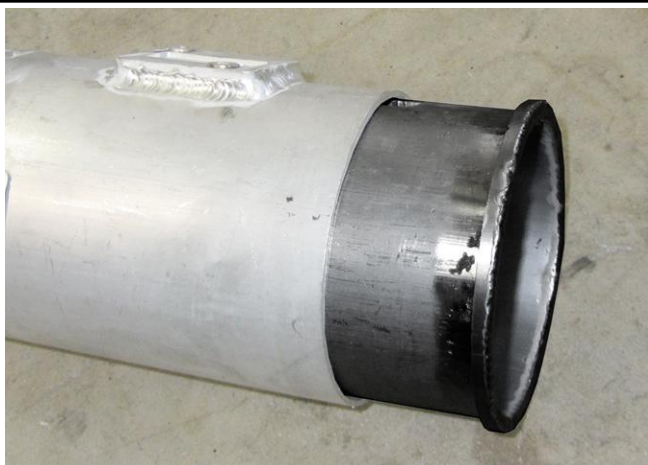
17. Install the MAF sleeve into the intake pipe as shown.
