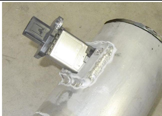
18. Once the MAF sleeve is lined up, remove the MAF sensor from the stock air box and install it onto the HPS intake pipe using the M4 screws included.
