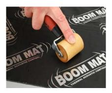
4. Once in the proper location, use your Boom Mat installation roller (050218) and apply pressure to ensure a strong bond between Boom Mat and the installation surface.
