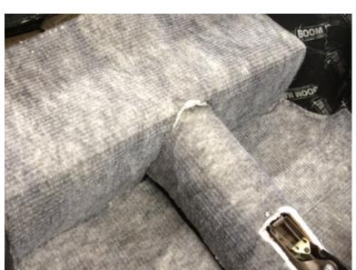
UC Lite installed with gray side up.
