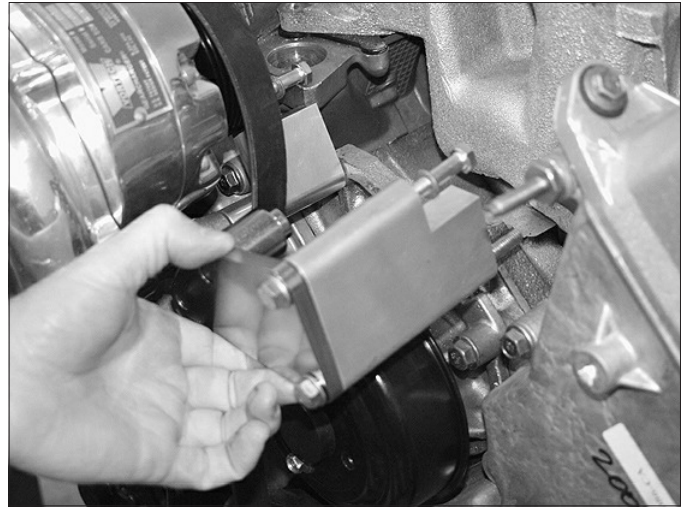
Fig. 8.2-g / Step 4 - Install alternator bracket 2 with idler plate assembly
