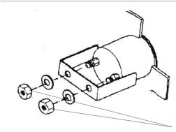
Do not over tighten bolts when installing U bracket. Doing so will cause damage to movement inside.
