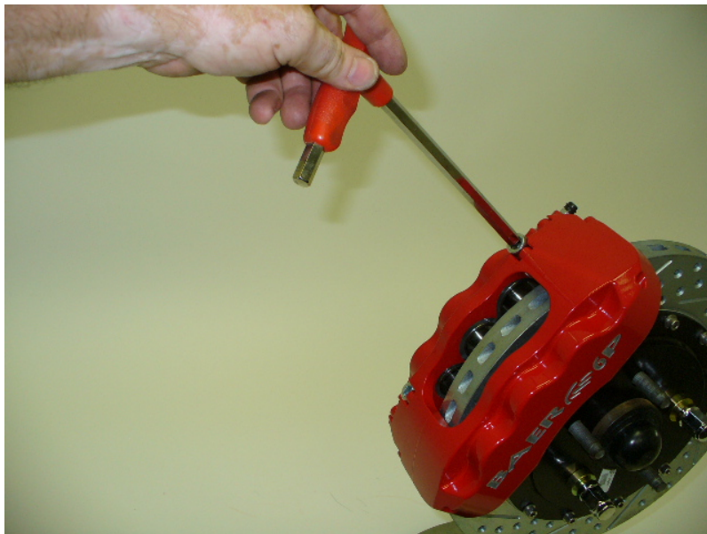
Install the caliper to measure clearance.
