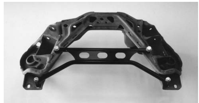
4-Point K-Brace placement on the K-member as viewed from the rear of the car
