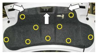
2. Cut out either the fastback or convertible template located in the back of this manual, depending on your application. Measure the scale on the template after printing it to ensure it is printed to the correct size. With the carpet removed, position the template on the bottom of the trunk lid. Use a center punch on the indicated areas to create locating marks for the bottom screws. Fastback bracket template shown below.
