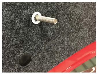
7. Install the spacers onto the studs overtop the carpet by turning them clockwise until the gap between the carpet and the spacer is closed.
