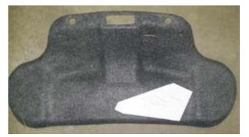
6. Install the carpet by reversing Step 1 and making sure to feed the studs on the mounting brackets through the cuts that were made in Step 5. Place the lock rings (W15X6X1-P-NF) on the studs.
