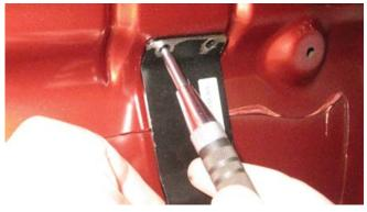
3. Use the mounting brackets to locate the top mounting holes and mark them with a center punch. Drill pilot holes at the center-punched locations using the 3/32" drill bit.
