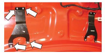
5. Cut out the provided fastback or convertible carpet template (1315-TRNKCRPT) found at the back of this instruction manual. Lay the template on the underside of the carpet. Make sure to line up the holes with the holes on the carpet for the push pins and pay attention to which side of the template is facing upward as it gets flipped for use on the driver side. Using a razor blade, cut an "X" into the carpet where the template shows. Passenger side fastback carpet template shown below.
