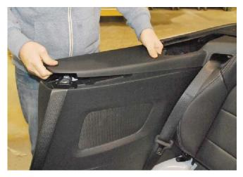
4. Disconnect the electrical connectors located behind the seat belt guides (if equipped) and remove the upper quarter trim panels.
