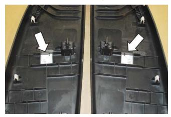
7. Using a center punch, mark the pilot hole locations as shown below.
