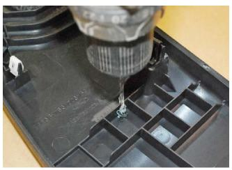
9. Turn the panels over and drill through the pilot holes with a 2" hole saw. If needed, apply masking tape to the surface to protect it from being damaged by the hole saw.
