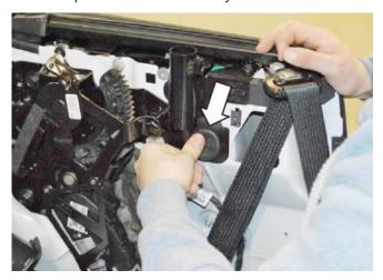
Reverse steps 10-11 of the disassembly section, in order to reinstall the speaker assemblies and quarter trim panels.
