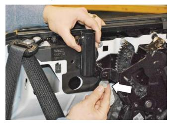
3. Install the one (1) 5/16" button head screw (P/N: 117000) and one (1) 5/16" serrated flange nut (P/N: 117001) into each bracket in the location shown below.
