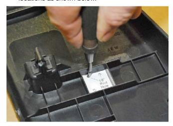
8. Drill the pilot holes with a 1/8" drill bit.
