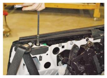
14. Remove one (1) 15 mm screw on each side of the vehicle as shown below.
