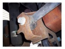
To the right is a picture of the passenger side panhard bar mount. The lower bolt is for the panhard bar, and the upper is for the support brace.
