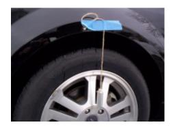
All you need is a string and a weight. Tie the weight to one end of the string. Hang the other end on the wheel well with tape. Make sure the weight is off of the ground, and not touching anything.
