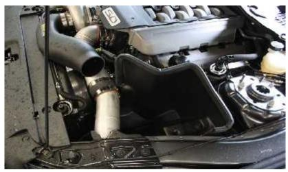
5 Install coupler – JLT Flow Tube – Filter on the tube coming from the blower and installation is complete.
